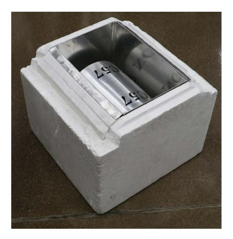
Figure 20-21. A neurocanister is immersed in liquid nitrogen in this styrofoam carrier when it is passed through a CT scanner.
