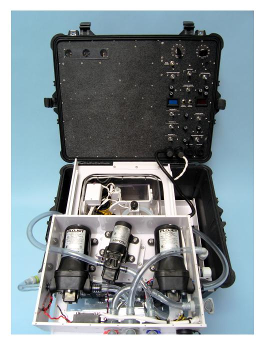
Figure 12-9. The pump boxfor LV3 was located on a platform that could slide out to allow access to the perfluorocarbon reservoir below. The whole assembly was designed to sit above the patient's legs on the rails of a portable ice bath, but its elevation greatly reduced the efficiency of suction from the lungs..
