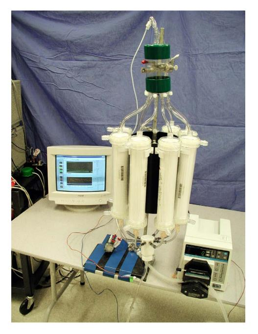
Figure 12-3. This cartridge system for cooling and oxygenating perfluorocarbon liquid was used experimentally for total liquid ventilation in 1996.
