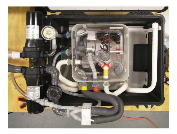
Figure 12-12. For LV4, a larger perfluorocarbon reservoir accommodated two subreservoirs, one to measure infusion volume and a second to measure the returned volume in each cycle, so that a running average could be calculated, indicating whether liquid was accumulating in the lungs. The additional sub-reservoir entailed complications such as a need for check valves and other associated plumbing. To
