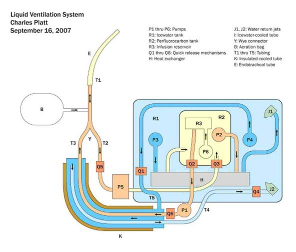
Figure 12-7. This diagram was created in preparation for a patent application filed in 2008. It shows the main components that were planned at that time for LV3, including the insulated delivery tube (K) with an icewater jacket, and external infusion and suction pumps (P1 and P5) to be mounted outside the Pelican container when the equipment was assembled.
