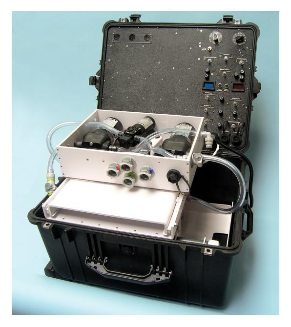
Figure 12-8. In LV3, batteries and chargers were were mounted inside the lid of the primary Pelican container, alongside switches and control electronics. A more powerful infusion pump and a more powerful suction pump than in LV2 were mounted in a separate box, together with a small pump that cooled an icewater jacket on the delivery tube (the tube is not shown here).
