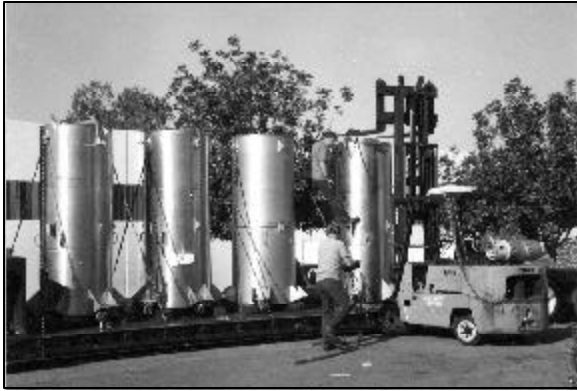
Bigfoot is loaded onto its flatbed truck with forklift; lifting was from the top.
